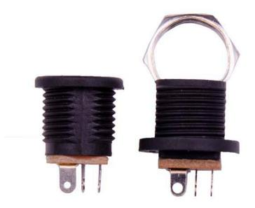
**Step 1:** Mount the AC adapter jack to the enclosure. Your kit may come with either an external thread or internal thread. Don't get confused by this. They still function exactly the same. You just thread the external nut on the outside and the internal nut on the inside. The picture below is of an internal nut jack.
