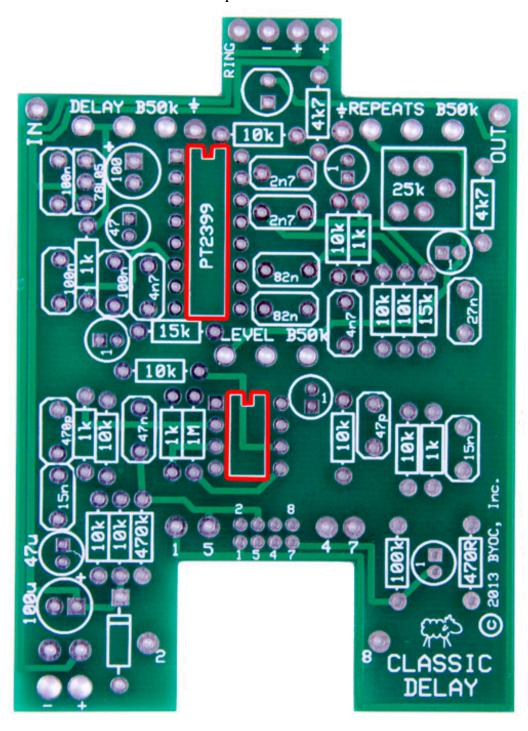
**Step 4:** Add the voltage regulator. Orient the 78L05 so that the flat side matches up with the flat side on the PCB layout.
