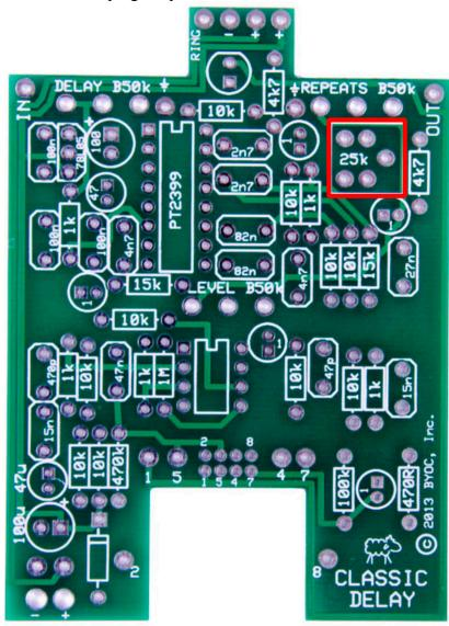
**Step 6:** Add the film capacitors. These are non-polarized so it can go in either direction.
