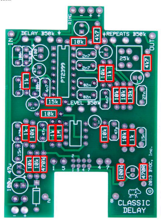
**Step 2**: Add the diode. Be sure to match the end of the diode with the stripe to the layout on the PCB. The striped end should go in the square solder pad.
