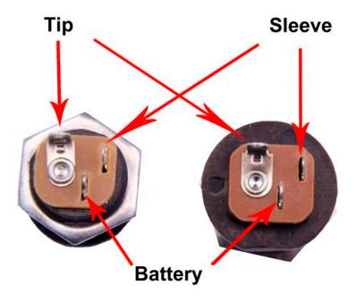
**Step 6:** Connect the TIP (negative) terminal of the DC adaptor jack to the eyelet on the PCB labeled "-". Connect the SLEEVE of the DC adaptor jack to the eyelet on the PCB labeled "+" farthest to the right. Connect the battery disconnect terminal of the DC adaptor jack to the second eyelet on the PCB labeled "+" located in the middle of the other two eyelets . See diagram on the next page.
