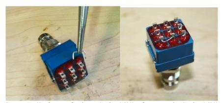
• Cut a 1.5" piece of wire. Strip 1/8" of one end. Strip 1/2" off the other end. Tin both ends. This will be used to connect lug/eyelet 4. The longer stripped end will be used to jumper lug 4 to 9.
