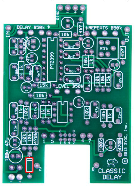
Step 3: Add the 16 pin and 4 pin IC sockets. ONLY SOLDER THE SOCKET! NOT THE ACTUAL IC! This is a socket. The sockets get soldered to the PCB. The ICs get inserted into the sockets. The actual IC chip itself, never gets soldered. You will insert the IC into the socket after the entire pedal has been built.
